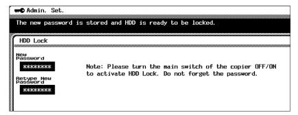
11 As instructed, turn the machine off, then on again. The hard disk is locked.
